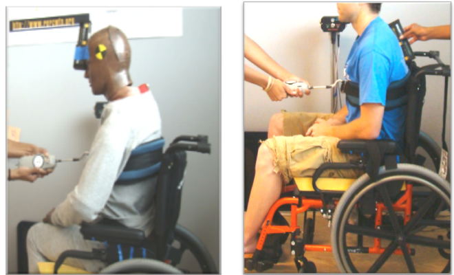
Figure 3 (left): The ATD is positioned and prepared with an inclinometer strapped to the head.
