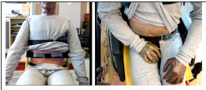
Figure 2: A Hybrid 2 ATD without (left) and with (right) the abdominal section in place.
